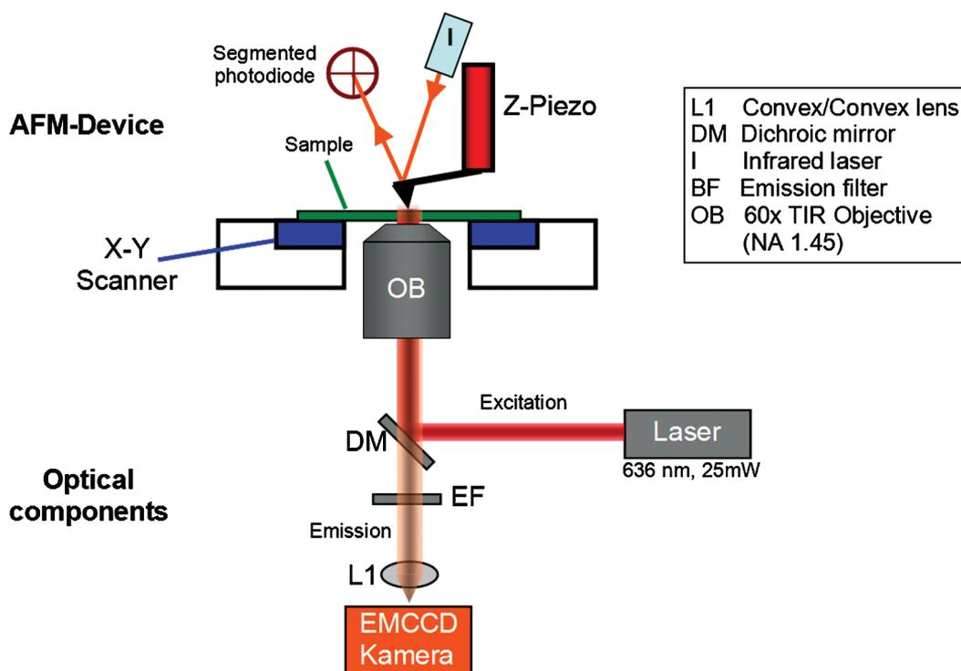
**Fig. S2.** Experimental combined Atomic Force Fluorescence Microscopy setup with TIRF excitation. The cantilever and the  $x$ - $y$  scanner movements are realized via precise piezos in nanometre range. The sample with the depot- and target areas on top is hold via a custom made aluminium support, which is fixed through magnets on the  $x$ - $y$  scan stage.
