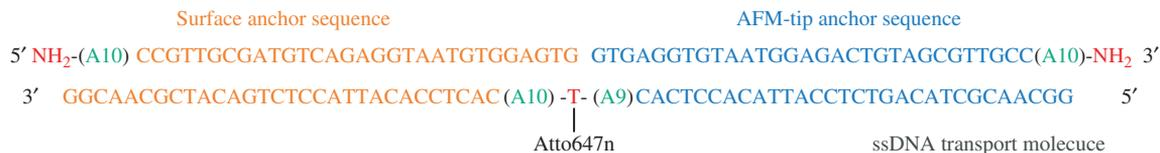
**Fig. S1.** Oligomers used in this transport study. The transfer ssDNA is 80 bases long and is modified with an Atto647n fluorophore at position 41-T (counted from 3'-end). The 30 bases long sequences at the AFM-tip side and on the surface are used to anchor the transfer ssDNA for both acquiring and deposition due to the partial complementarities to the transfer ssDNA molecule. All oligomers were synthesized and purified (HPLC-grade) from Purimex (Grebstein, Germany).
